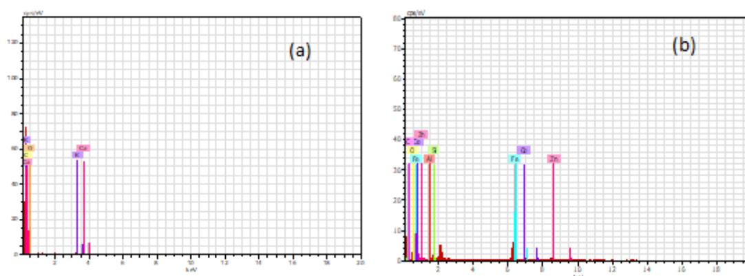
**Figure 4: The results of the SEM-EDX spectrum on the adsorbent are (a) activated carbon and (b) magnetic activated carbon**
