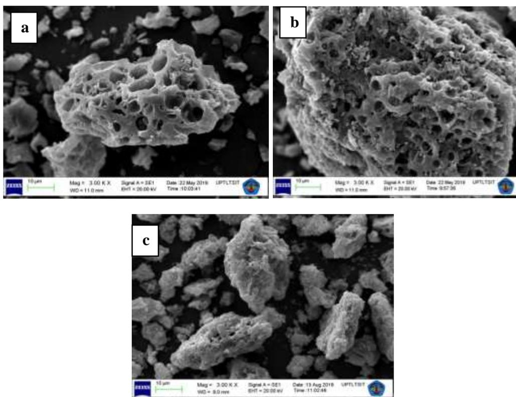
**Figure 3: Results of SEM micrographs of the samples investigated: (a) inactivated carbon, (b) activated carbon and (c) magnetically activated carbon**
