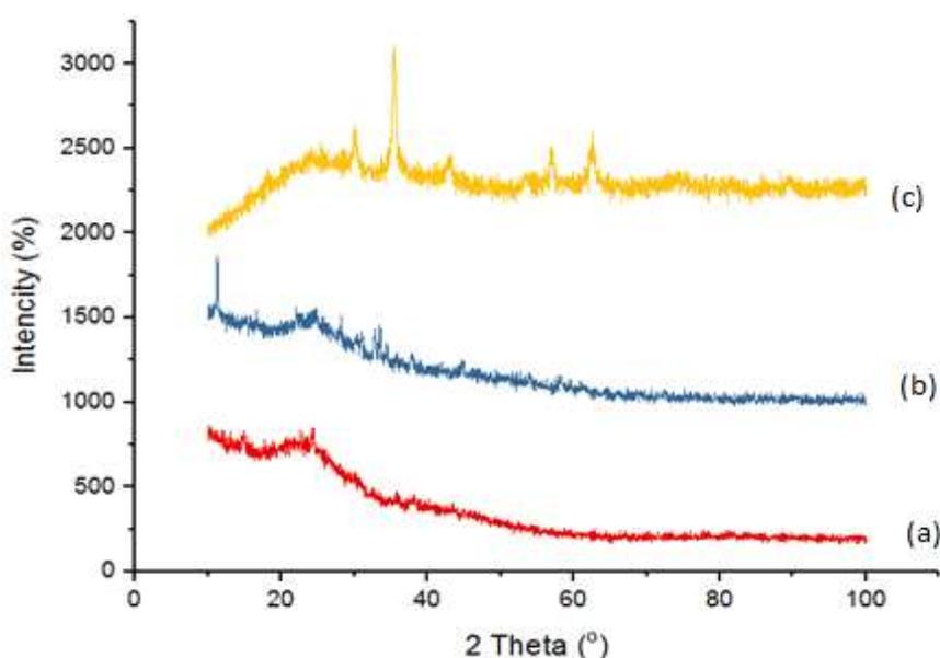
Figure 5: XRD diffractograms samples investigated: (a) inactivated carbon, (b) activated carbon and (c) magnetic activated carbon
